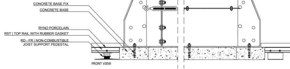
**TERRASMART RAIL PAVING SYSTEM IGNO - LATTICE FRAME**
