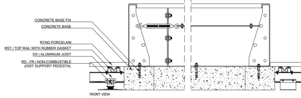
**CONCRETE FIXING DETAIL FOR VARIOUS RYNO DECKING SYSTEMS**
