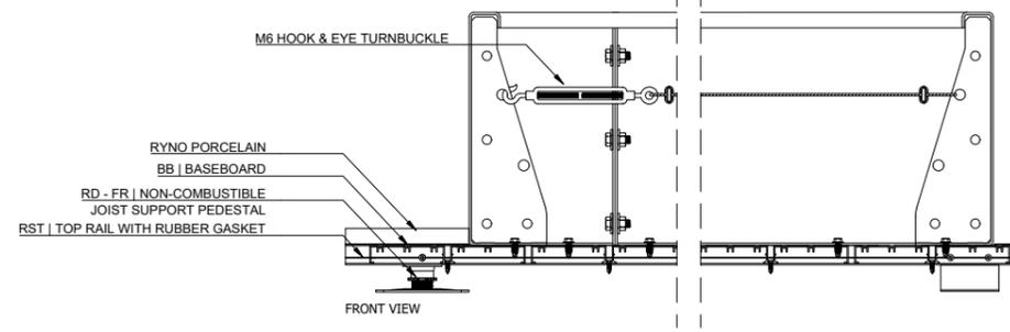
**TERRASMART RAIL PAVING SYSTEM IGNO - LATTICE FRAME**
