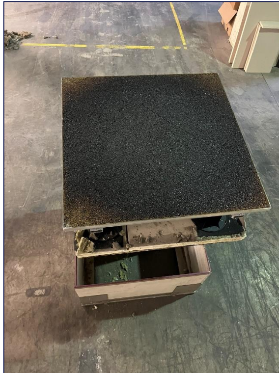
Figure 14: Damage investigation – Sample G – After 60 min of radiant heat exposure.
