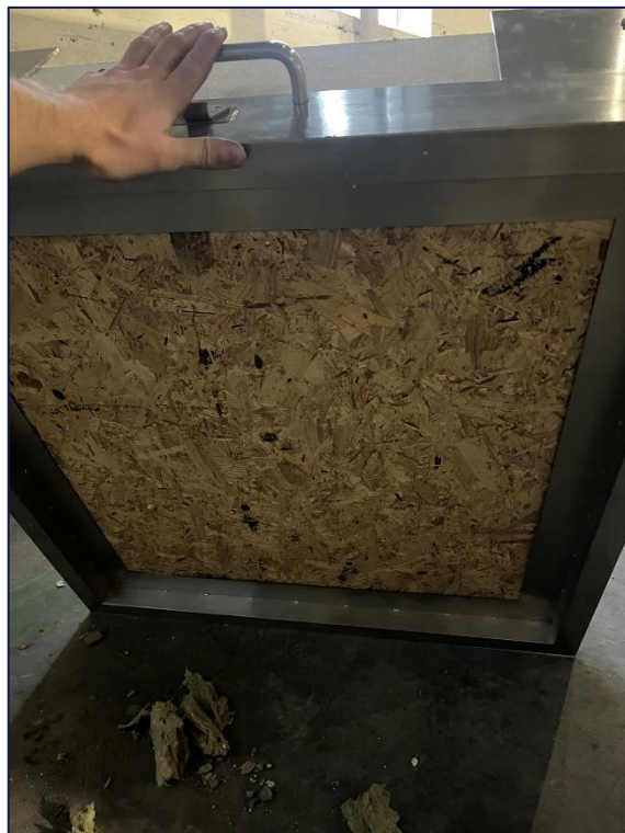
Figure 9: Damage investigation – Sample C – Non-exposed side of the specimen.
