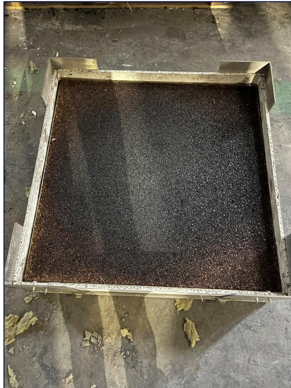
Figure 8: Damage investigation – Sample E – After 60 min of radiant heat exposure.
