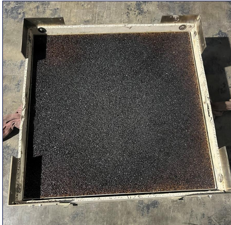
Figure 11: Damage investigation – Sample F – After 60 min of radiant heat exposure.
