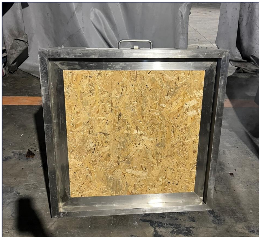
Figure 12: Damage investigation – Sample F – Non-exposed side of the specimen.
