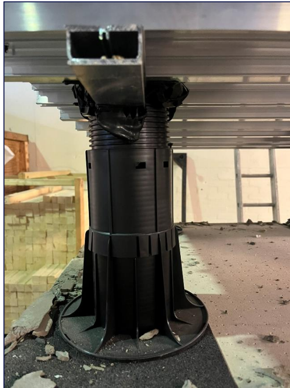
Figure 16: Damage investigation – Sample G – Pedestal.
