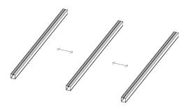
2. Lift joists on to pedestal supports at each end of joist and level up. Fig B
